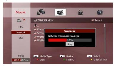
You can also scan for a specific network device. Press the **GREEN** button, enter the IP address of the device and select "OK".
