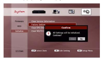
Select "Yes" and press the **OK** button to proceed. To cancel the factory setting function, select "No" and press the **OK** button, or press the **EXIT** button.
