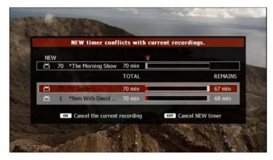
In order to allow the timer to begin, you must stop one of the current recordings. Use the **UP/DOWN** buttons to select a recording and press **OK** to stop that recording. If you don't wish to stop either of the current recordings, press **EXIT** to cancel the pending timer.
