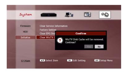
Select "Yes" and press the **OK** button to proceed. To cancel the clear WizTV disk cache function, select "No" and press the **OK** button, or press the **EXIT** button.
