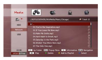
To choose a particular selection of files, select a desired file and press the **BLUE** button. A tick will appear in the box alongside the selected file. Repeat this procedure for the remainder of your selection.
