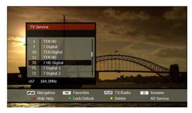
The service list window is titled "TV Service" or "Radio Service", depending on which service mode you are currently using, and will list all available TV or radio services accordingly. Select a service by using the **UP/DOWN** buttons, and press the **OK** button to change to that service.
