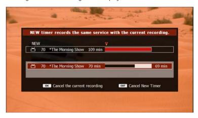
In order to allow the timer to begin, you must stop the current recording by pressing the **OK** button. If you don't wish to stop the current recording, press **EXIT** to cancel the pending timer.
