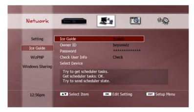
• Ice Guide: Select "Enable" to allow the DP-Lite to get and update the electronic program guide (EPG) from the IceTV service. If you select "Disable", the DP-Lite will only update the EPG with the data supplied by the broadcaster of the currently viewed service.
