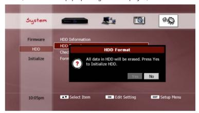
Select "Yes" and press the **OK** button to proceed. To cancel the HDD format function, select "No" and press the **OK** button, or press the **EXIT** button. If you select "Yes", the DP-Lite will restart and format the internal HDD automatically.
