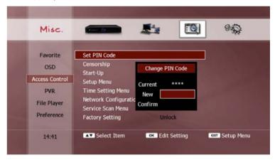
Use the **NUMERIC** buttons to enter the current PIN number, then your desired new PIN number, and then repeat your desired new PIN number to confirm it was entered correctly
