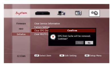
Select "Yes" and press the **OK** button to proceed. To cancel the clear IceGuide disk cache function, select "No" and press the **OK** button, or press the **EXIT** button.
