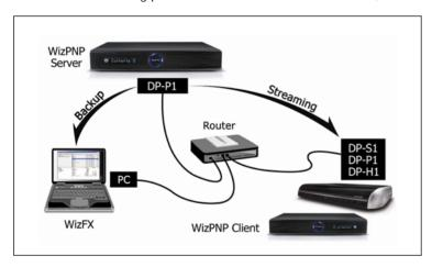
You can set the DP-Lite to be a WizPNP client, a WizPNP server, or both client and server simultaneously.
