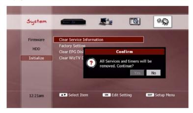
Select "Yes" and press the **OK** button to proceed. To cancel the clear services function, select "No" and press the **OK** button, or press the **EXIT** button.
