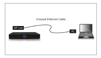
If your PC has the DHCP server feature and it is enabled, all the configurations for networking will be set automatically and the DP-Lite is ready to communicate with your PC. If your PC does not have the DHCP server feature, you must disable the DHCP feature and set IP (Internet Protocol) information manually for the DP-Lite and PC. For more information on manually configuring DHCP, please refer to Chapter 4 "Quick Setup".
