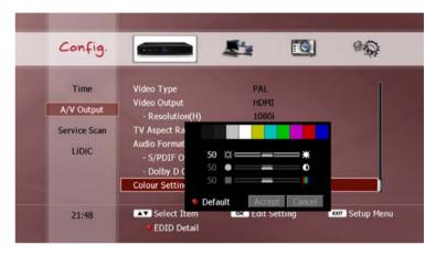
The three options are brightness, contrast and saturation. Use the **UP/DOWN** buttons to select each option, and adjust the setting with the **LEFT/RIGHT** buttons. You can restore all colour settings to the factory default values by pressing the **RED** button. To apply your chosen settings, use the **UP/DOWN** buttons to select "Accept" and press **OK**. To cancel the new settings, select "Cancel" and press **OK**, or press the **EXIT** button.
